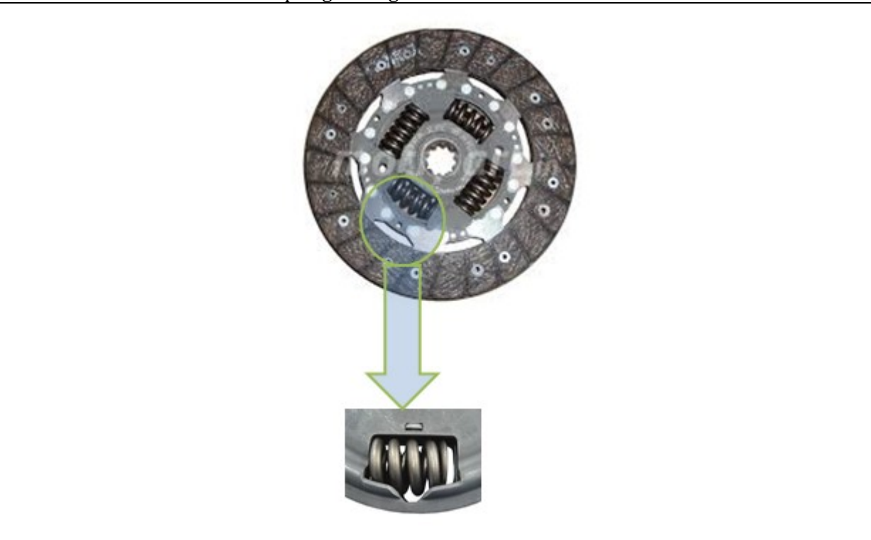
Illustration 2: Clutch Plate and Spring Arrangement for Torsional Vibration Isolation
